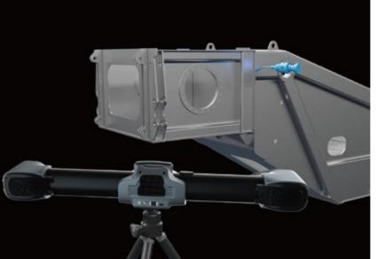
Its i-Tracker can be combined with tool simulators and path planning software to form M-Track, an intelligent robotic path planning and guiding system. The system comprises perception, planning, and execution modules, which cater to different applications such as grinding, coating, welding, and more.
